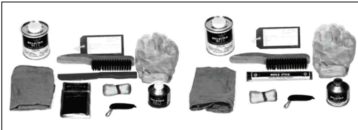
Figure 4-1. Hull and metal component repair materials
