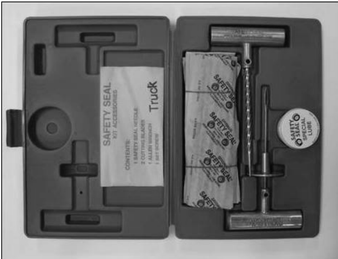
Figure 4-6. Tire patch materials and tire plug kit
