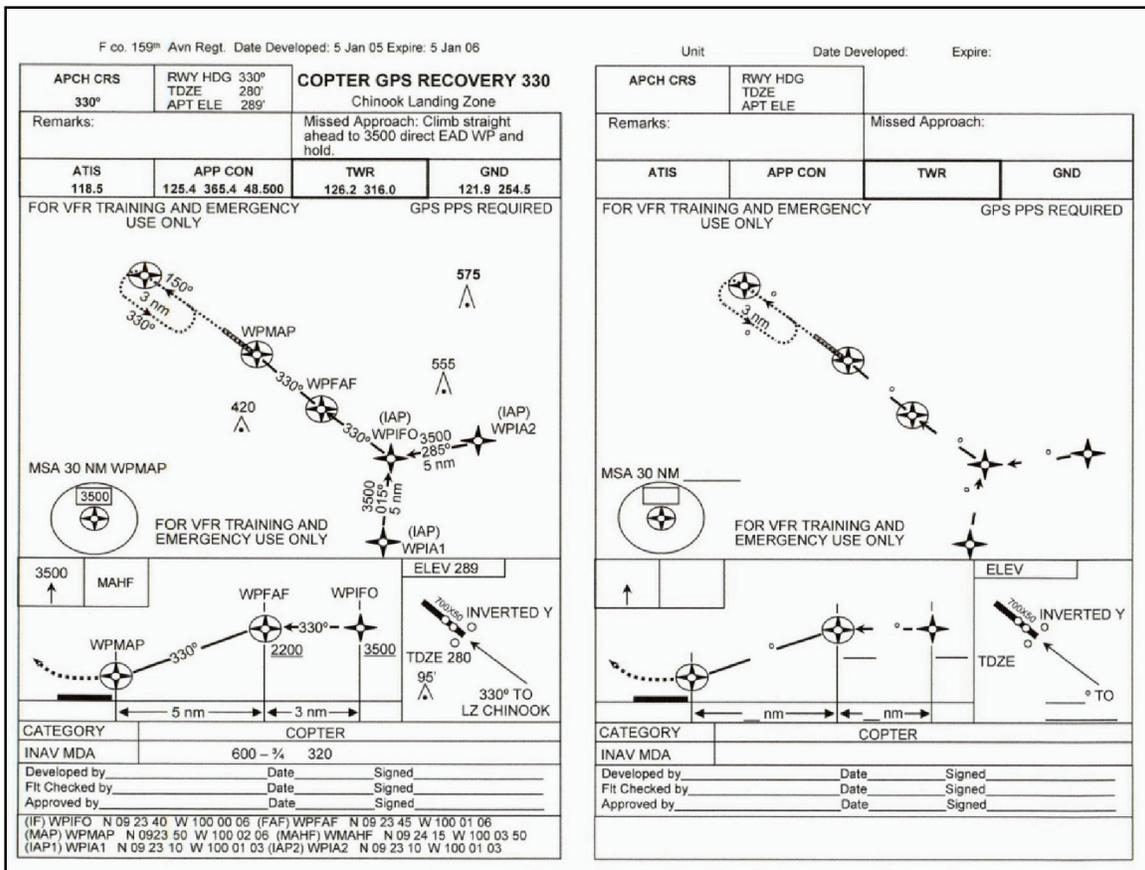
Figure 4-10. Sample of emergency GPS diagram
