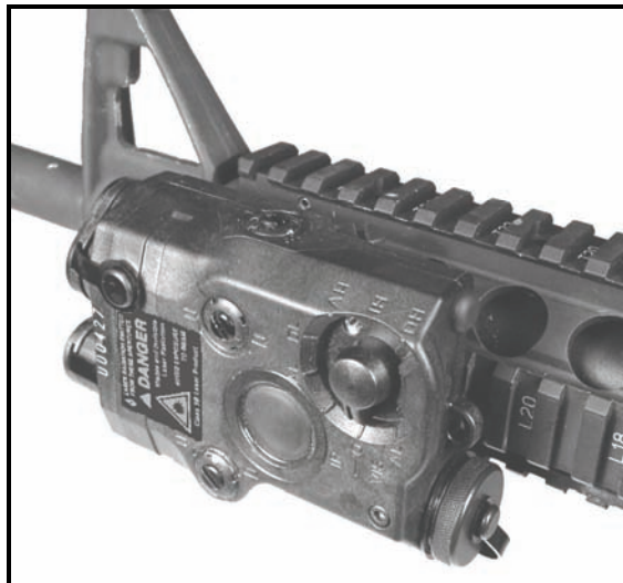
Figure 2-34. AN/PEQ-15 mounted on M4 carbine.
