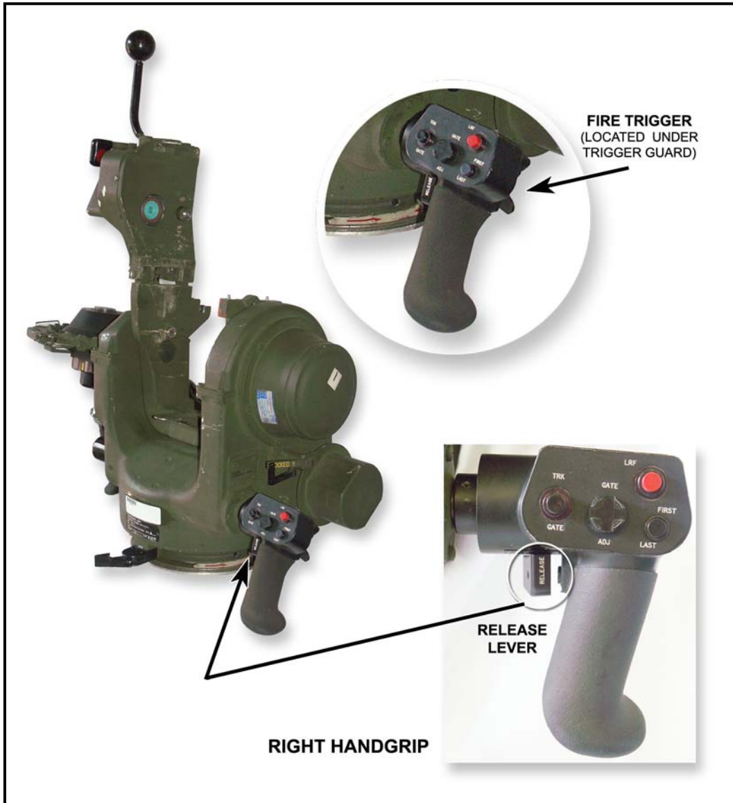
Figure 2-18. Release lever (right handgrip) and fire trigger.
