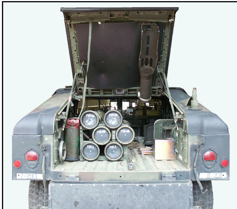
Figure 3-18. Launch tube stowed on cargo shell door.
