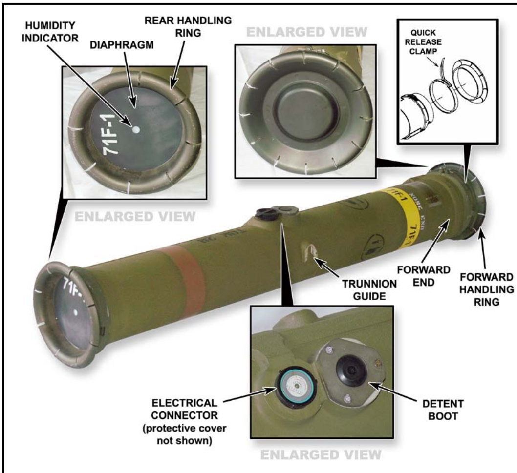
Figure 1-14. Encased missile components.
