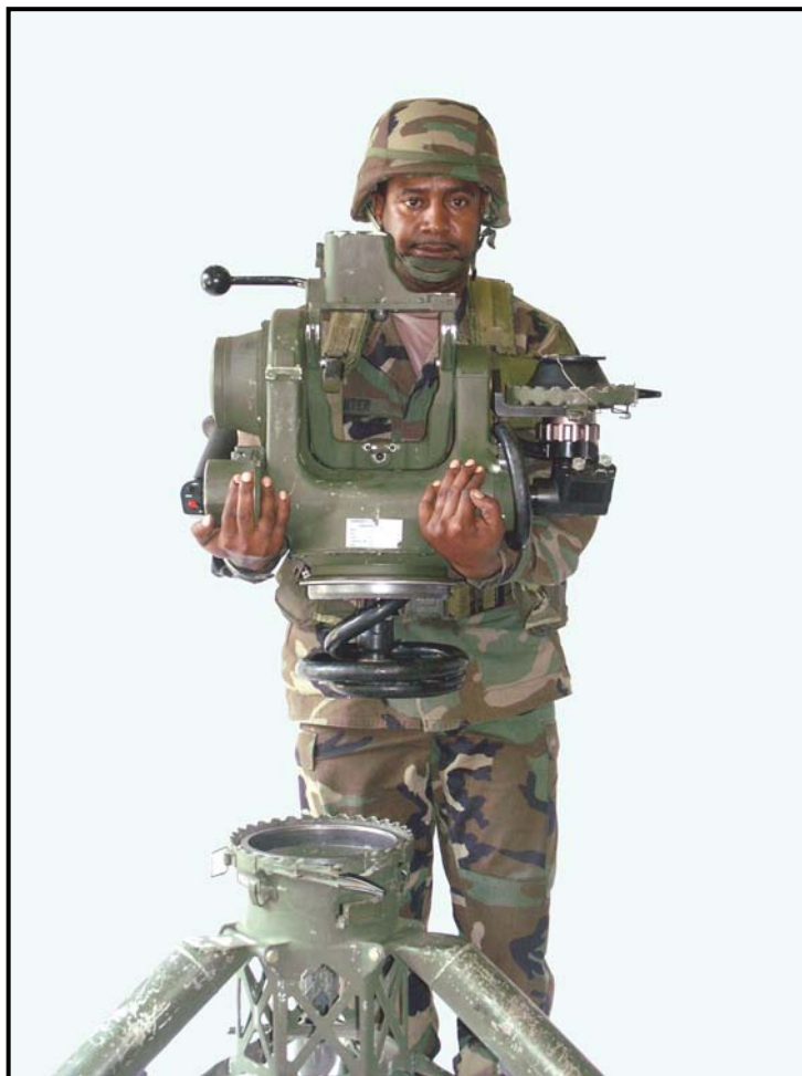
Figure 3-22. Removing the TU from the tripod.
