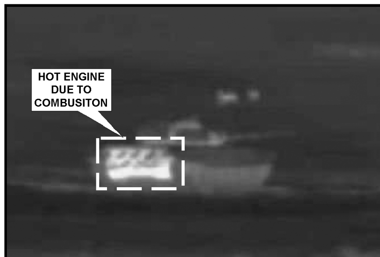
Figure C-3. Heat caused by combustion.
