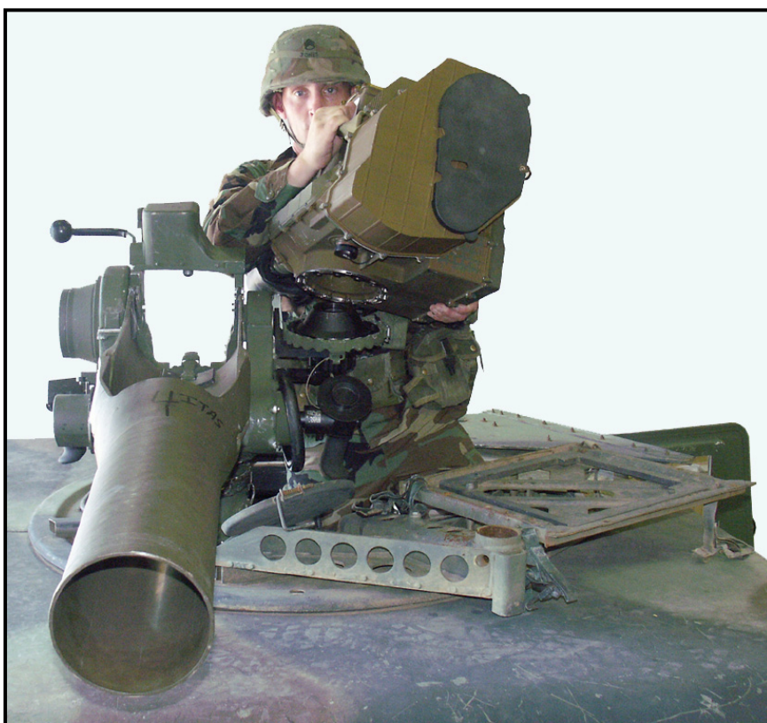
Figure 3-5. TAS being placed on TAS mount, window forward.
