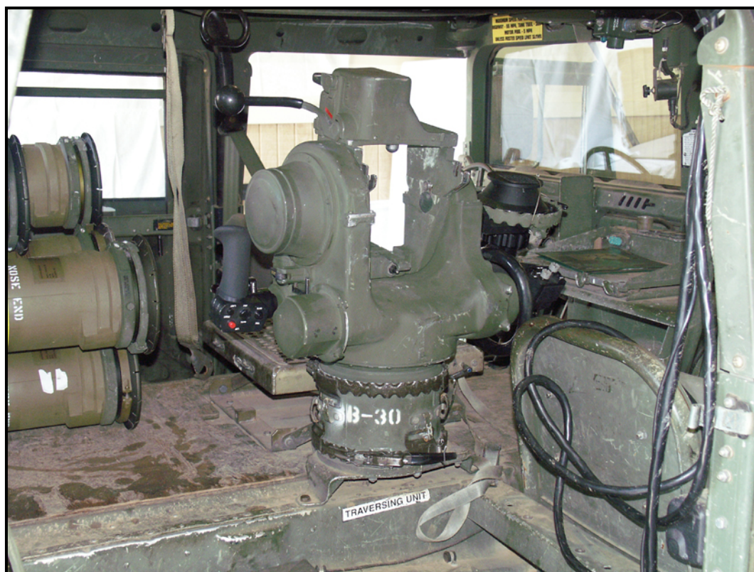
Figure 3-23. TU stowed on the TU adapter.
