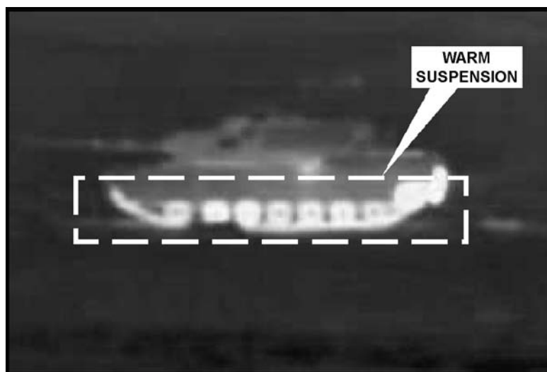
Figure C-4. Heat caused by friction.
