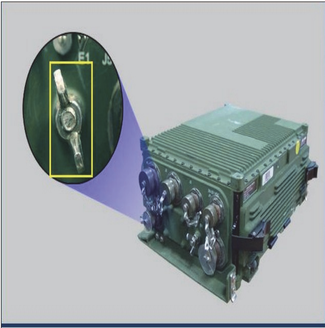
Figure 3-32. Hand tighten ground strap thumbscrew.
