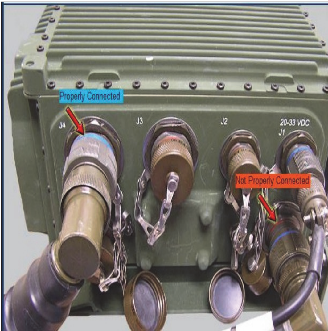
Figure 3-34. Check cables, connectors and mounting hardware for any damages.
