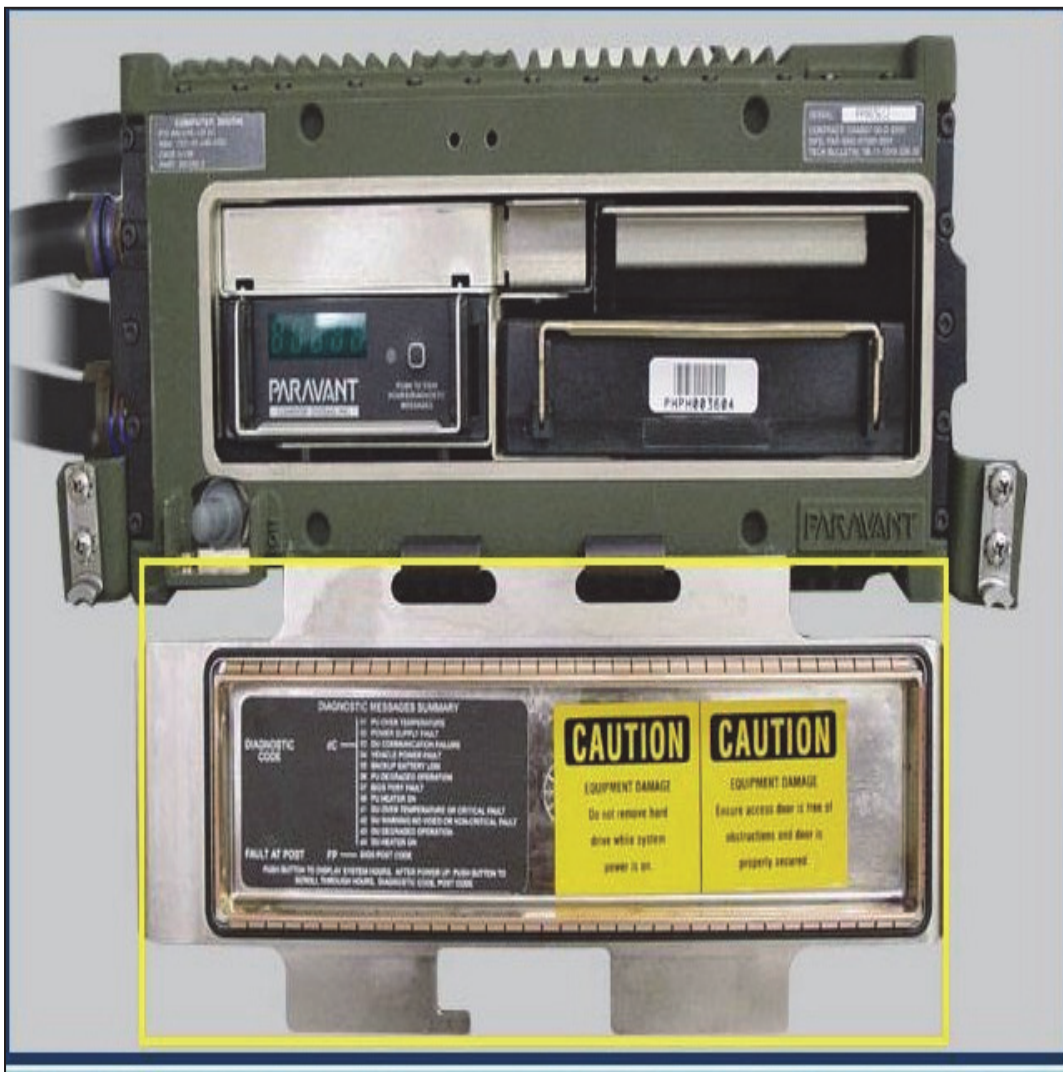
Figure 3-38. Check the Processor Unit for any obstruction, bad seal, broken, missing or loose capture fasteners.
