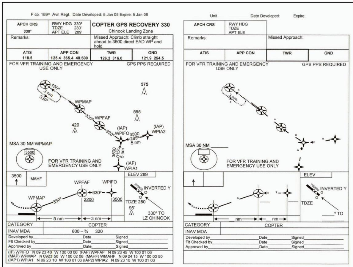
Figure 4-10. Sample of emergency GPS diagram
