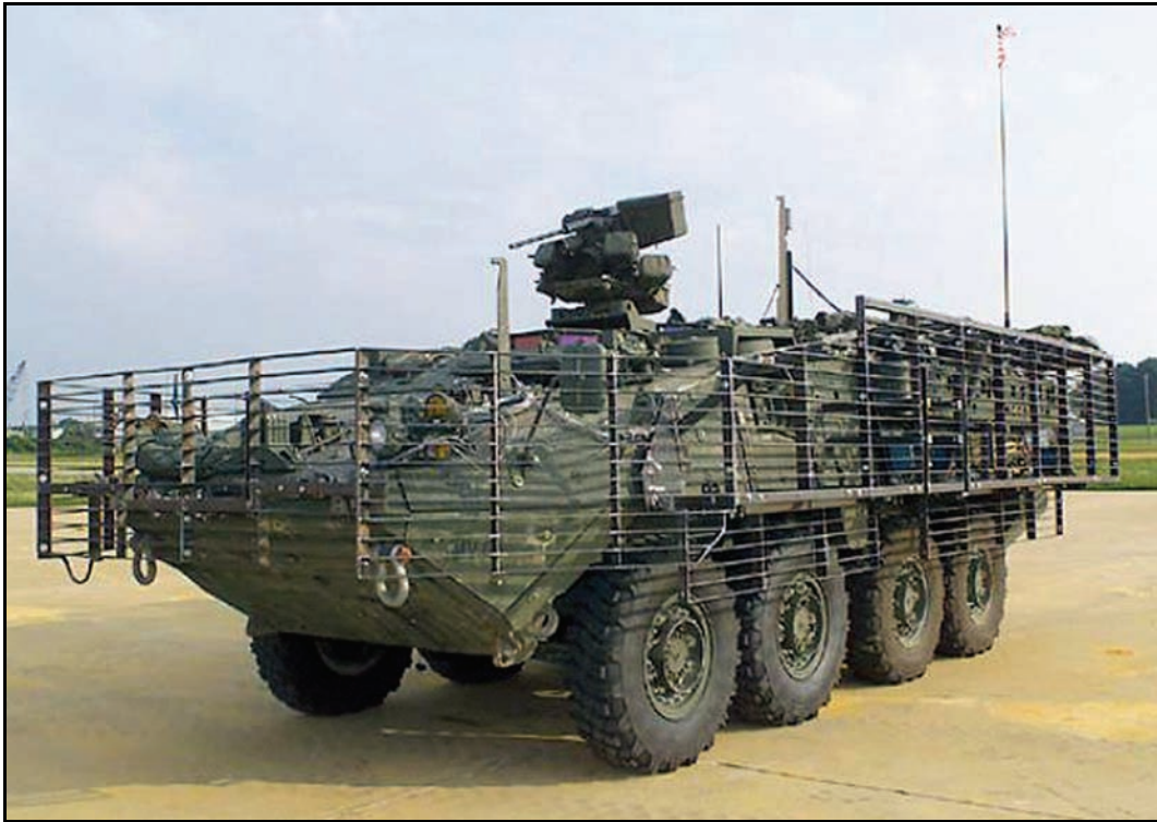
Figure 8-1. Slat armor package.
