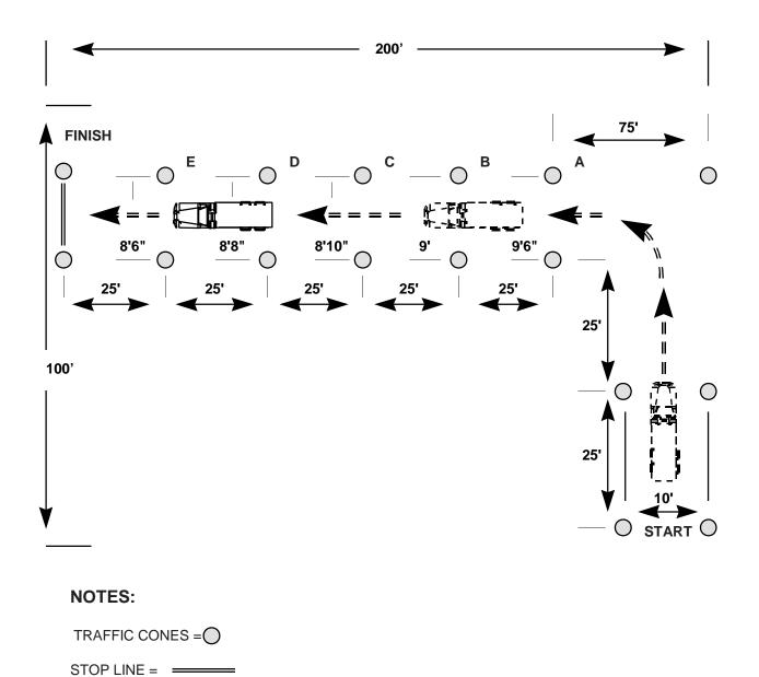
Figure 6-2. 5-ton cargo diminishing clearance
