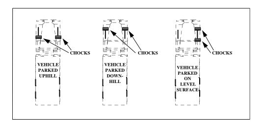
Figure 4-12. Correct chock block placement
