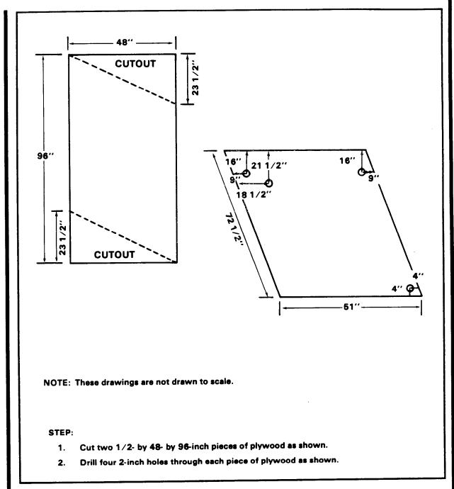
Figure 4-36. Parachute protector boards prepared
