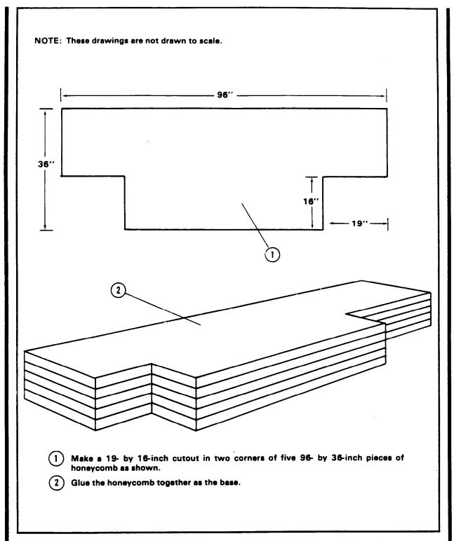
Figure 4-3. Stacks 1 and 12 prepared
