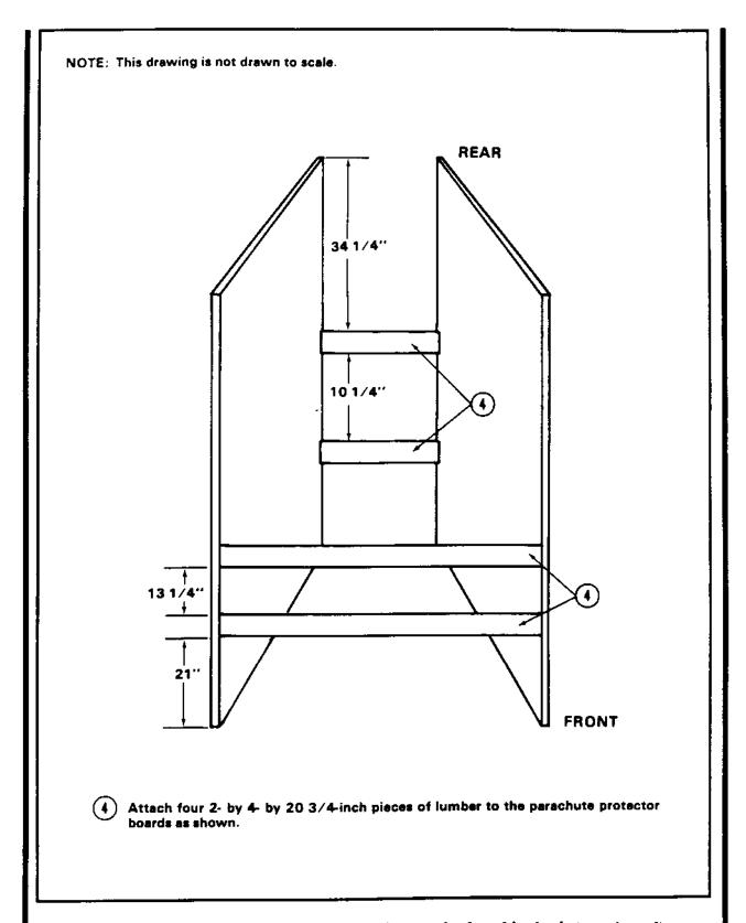
Figure 4-37. Parachute protector boards attached and lashed (continued)
