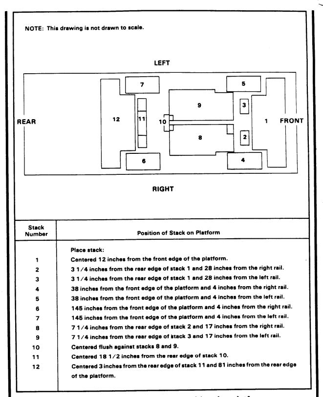
Figure 4-10. Honeycomb stacks positioned on platform
