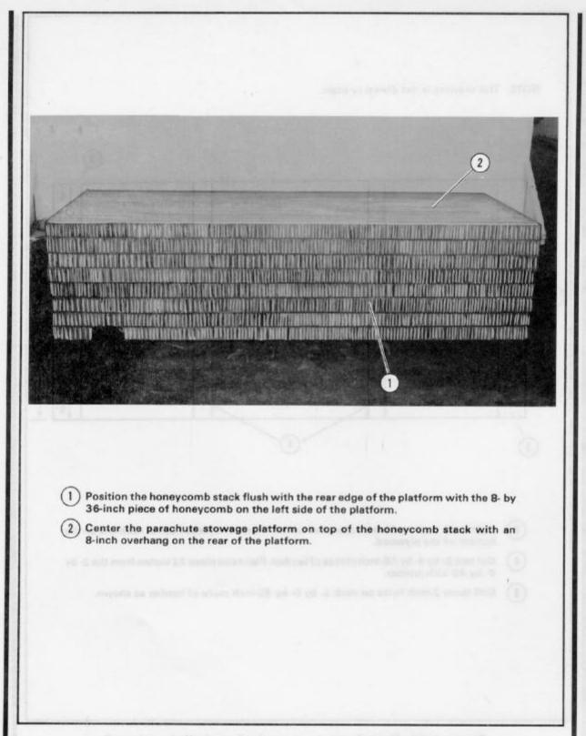
Figure 4-34. Honeycomb stack and parachute stowage platform positioned
