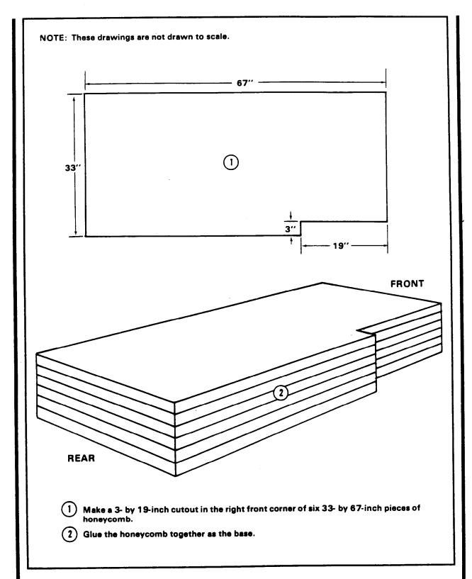
Figure 4-6. Stack 8 prepared
