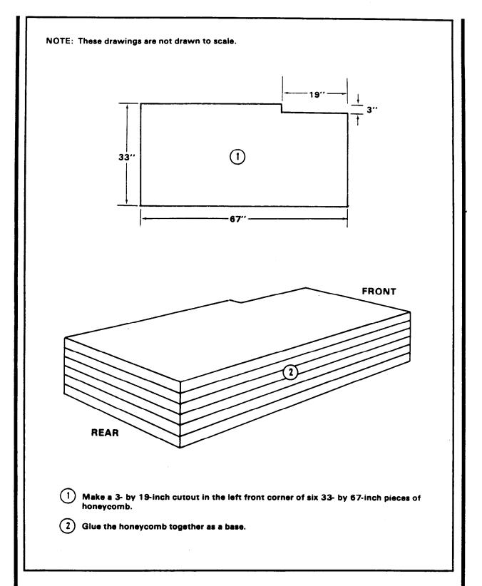
Figure 4-7. Stack 9 prepared
