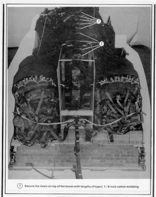
Figure 4-46. M-2 release installed (continued)
