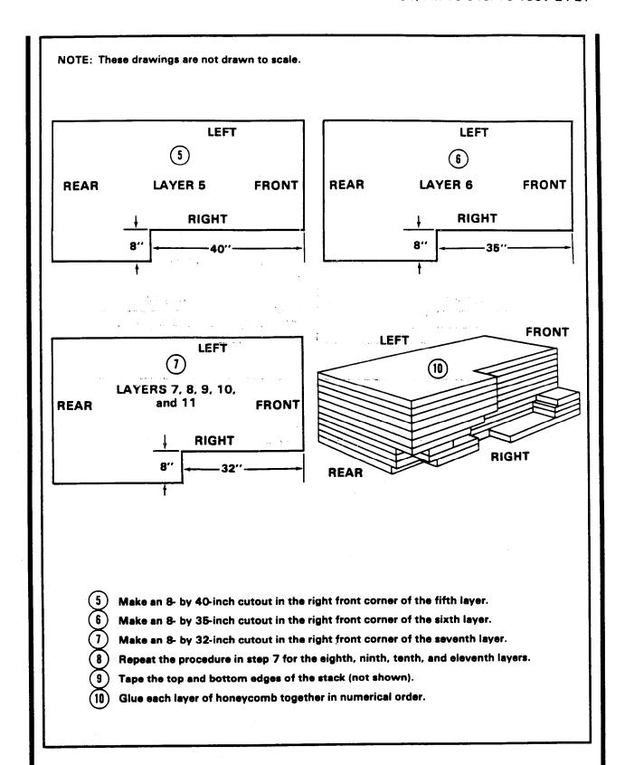
Figure 4-24. Parachute release support prepared (continued)
