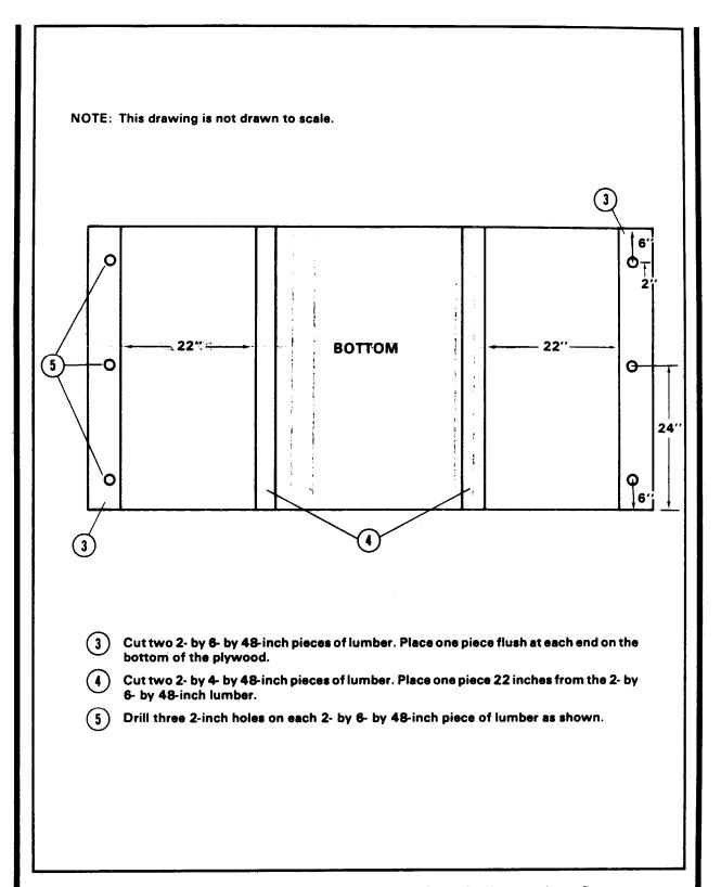
Figure 4-33. Parachute stowage platform built (continued)
