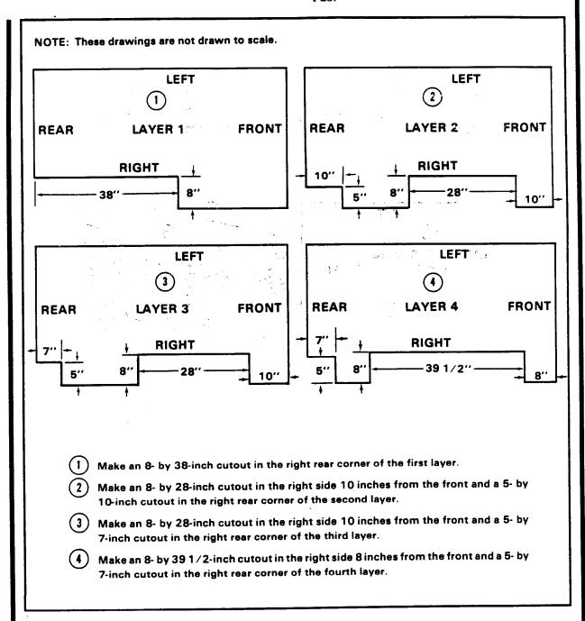
Figure 4-24. Parachute release support prepared
