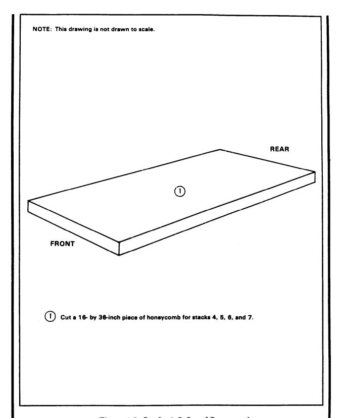
Figure 4-5. Stacks 4, 5, 6, and 7 prepared
