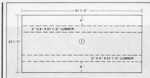
Construct a support tray for the storage box on the left side of the crane as shown above using 3/4-inch plywood and sixpenny nails.
