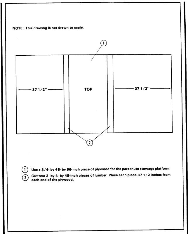
Figure 4-33. Parachute stowage platform built
