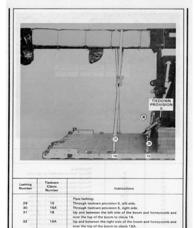
Figure 4-31. Lashings 29 through 32 installed
