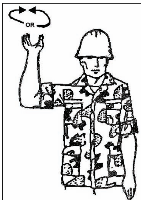
Figure 3-88. Lock/Unlock Tophandler Bayonet Locks
